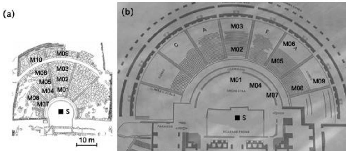
Figure 2. Sound source (S) and receivers (M01-M10). (a) Delphi; (b) Taormina.
