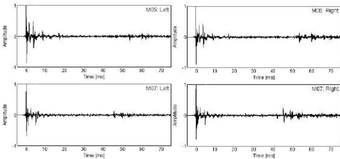
Figure 3. Binaural impulse responses as typical examples of the measurements.
