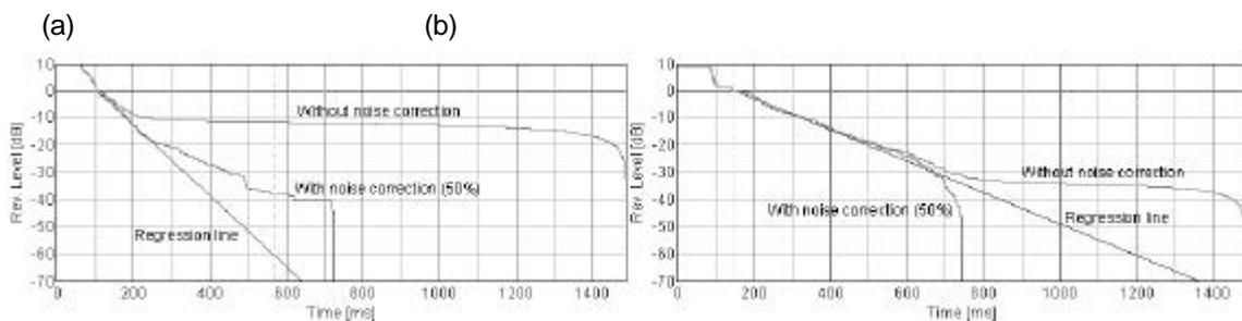
Figure 4. Decay curves for reverberation obtained by Schroeder's method as typical examples of the measurements. (a) Delphi (at M05) (b) Taormina (at M07).
