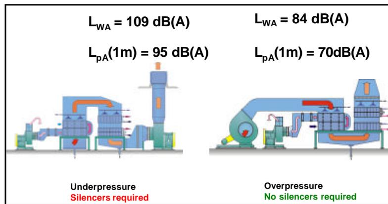
Figure 2. Heat recovery stacks, underpressure and overpressure.
