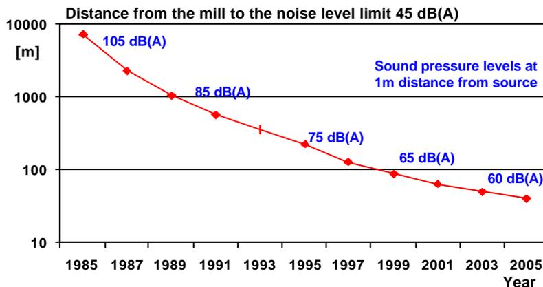
Figure 1. Distance to the equivalent SPL of 45 dB(A) in 1985-2005.
