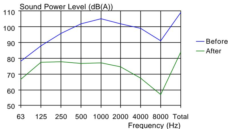
Figure 3. Sound power level before and after a heat recovery stack.
