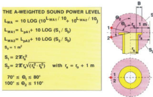
Figure 4. Sound level measurement DIN 45 635-47-KL3.
