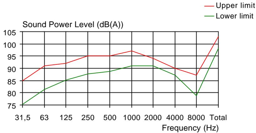
Figure 7. Total attenuated sound power level of PM ventilation.
