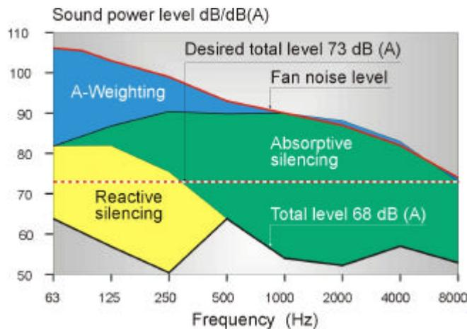
Figure 5. Fan noise attenuation (exhaust air).
