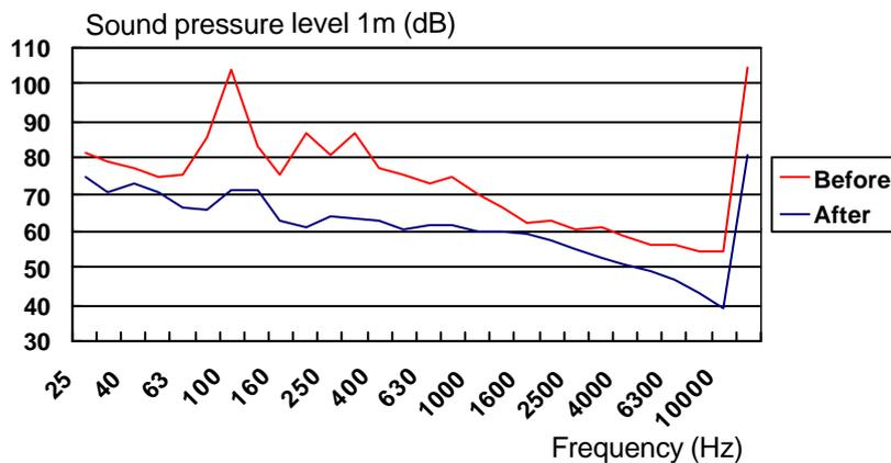
Figure 9. Sound pressure level before and after silencer installation.
