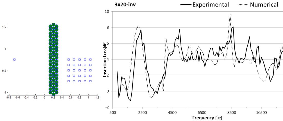
Figure 2 – Geometrical setup and sound attenuations (experimental vs. numerical)
