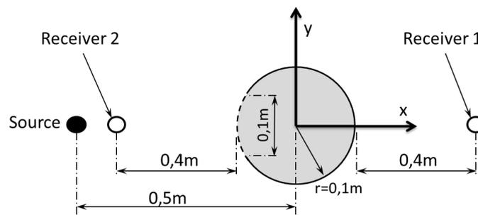
Figure 3 – Geometrical setup for MFS and BEM based numerical models analysis
