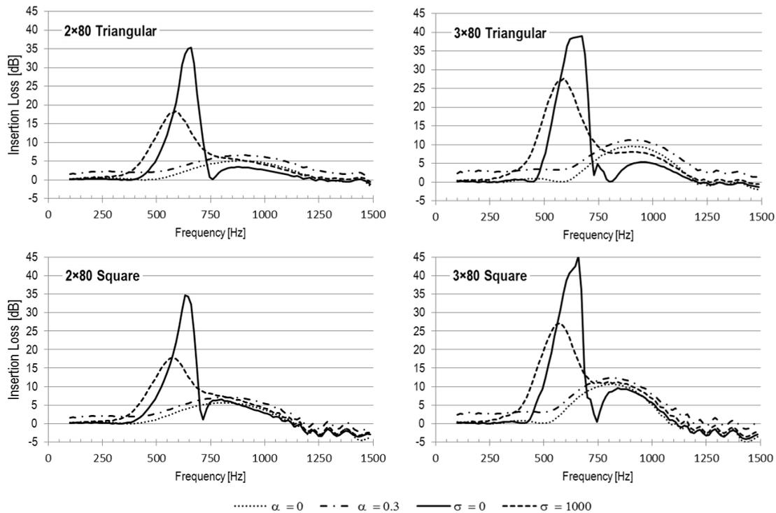
Figure 6 – Sound attenuations [dB] for different SC geometries and types of scatterers.
