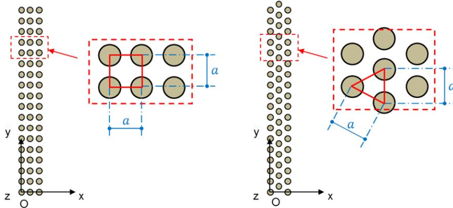
Figure 5 – Square and triangular lattice configurations of the Sonic Crystal barriers.
