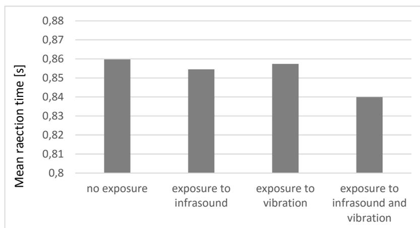
Figure 2 – Comparison of test results carried out with the use of the STD Simulator (no statistically significant variation at  $p < .05$ )
