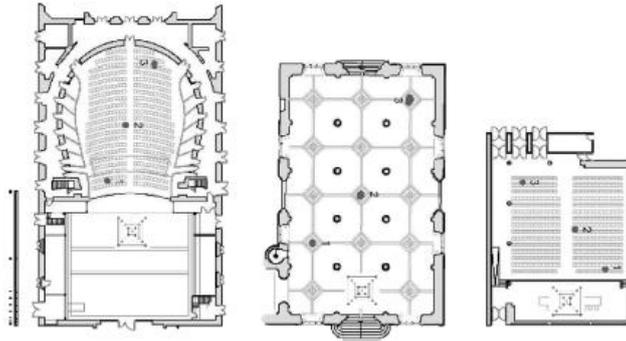
Figure 4. Receivers where auralizations were computed together with source position (represented as shown in Fig. 3). From top to bottom: Paranimf, Lonja, and Principal Theater of Valencia.
