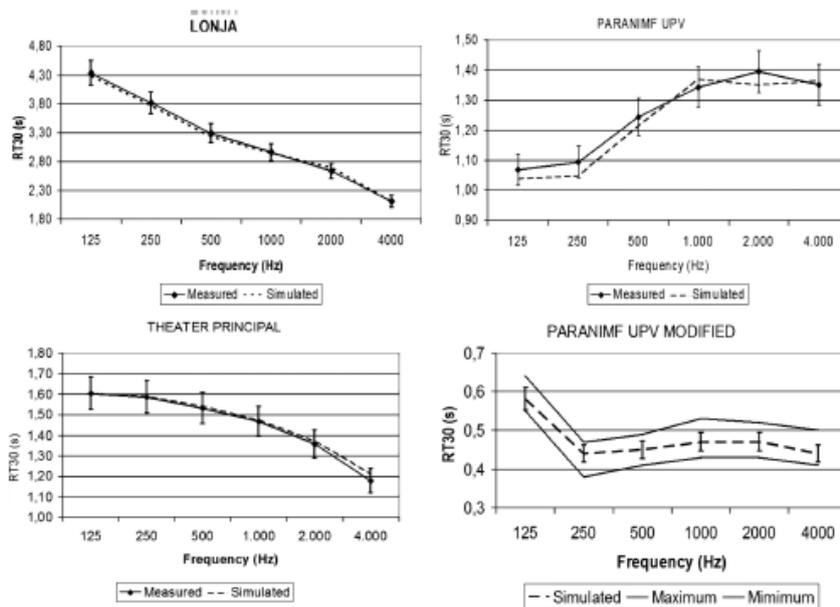
Figure 2. RT30 calibration in each room. In the modified Paranimf, the simulated RT30, together with its range, is shown.
