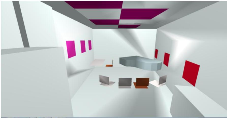
Figure 7 – Test room with additional 3 low freq. and 5 medium freq. absorbers on the walls.
