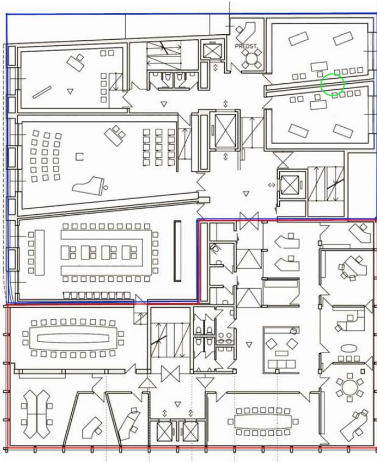
Figure 2 – Plan of the 3<sup>rd</sup> floor of the new building [12]. The old office building is shown in red, and the newly added part in blue. The green circle indicates a detail of a double wall construction.
