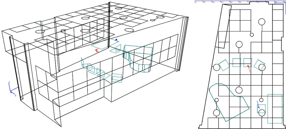
Figure 4 – Test room used for auralization. The number and position of acoustic elements were varied (type 1 – type 6).
