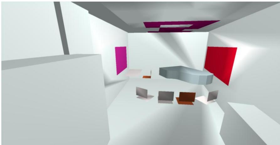
Figure 9 – Test room with 15 binary diffusers, 6 low freq. and 10 medium freq. absorbers, all grouped around the listener and the musician.
