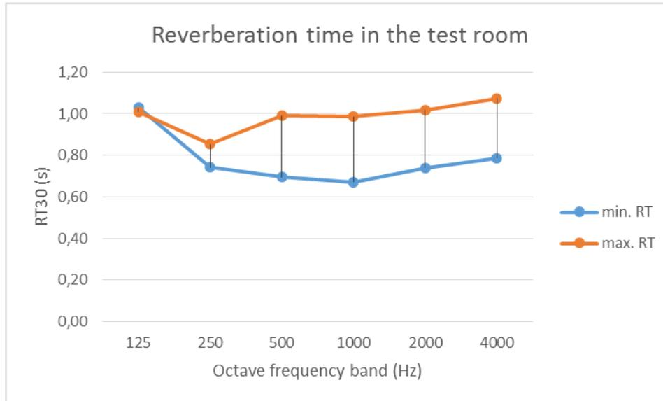
Figure 12 – Variations of the reverberation time in the test room with changeable acoustic elements.
