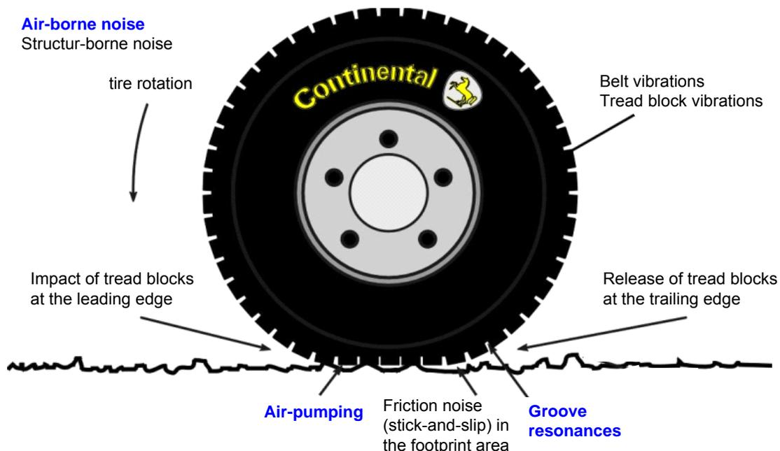
**Figure 1. Tyre schematic indicating the main excitation mechanisms upon the interaction of the tyre with the road surface.**
