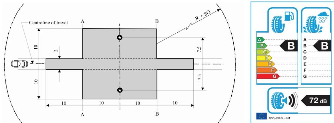
**Figure 2. Left: a highly schematic representation of the noise coast-by test [9]. The shaded part represents the test area that is passed by the test vehicle. Two microphones are mounted, each ( $7.5 \pm 0.05$ ) m away from the reference line (centre line of the test track) and ( $1.2 \pm 0.02$ ) m above the ground. Source: Directive 2001/43/EC [2]. Right: example of a label for a C1 class tyre. Source: Reg. 122/2009 [8].**
