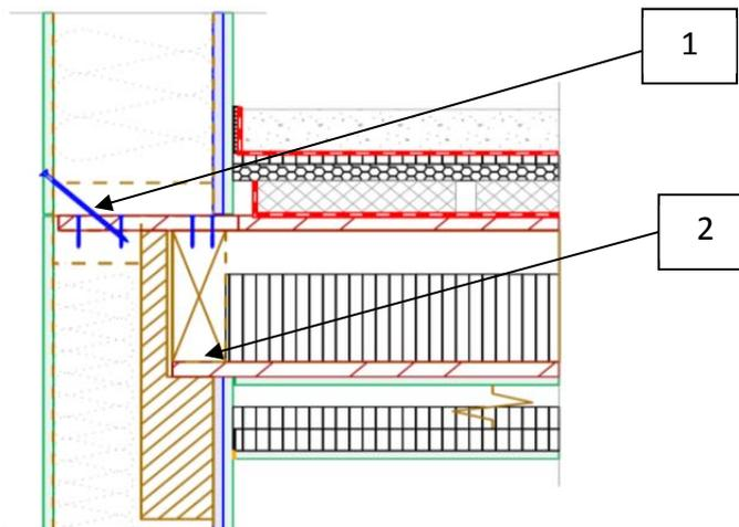
Figure 1. Basic construction of test junction indicating where the resilient layers have been introduced.
