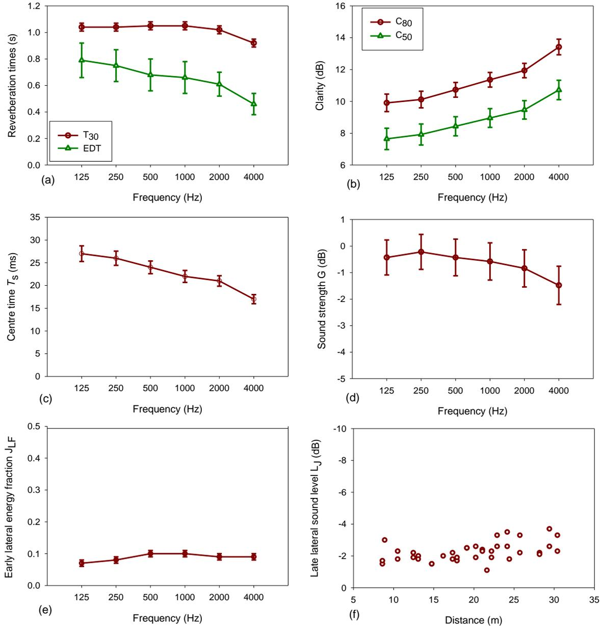
Figure 5 – Simulated monaural acoustic parameters in the Roman theatre of Malacca: (a) Reverberation time parameters,  $T_{30}$  and EDT; (b) Clarity parameters,  $C_{80}$  and  $C_{50}$ ; (c) Centre time,  $T_S$ ; (d) Sound strength,  $G$ ; and (e) Early lateral energy fraction,  $J_{LF}$ , all as a function of frequency. (f) Late lateral sound level,  $L_J$ , energy averaged as a function of source-receiver distance.
