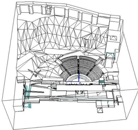
Figure 3 – Section of the final geometric model of the theatre.
