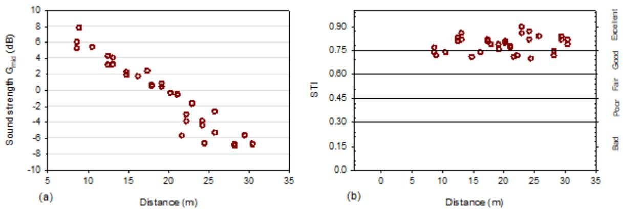
Figure 7 – (a) Sound strength  $G_{mid}$ , and (b) STI parameters versus source-receiver distance.
