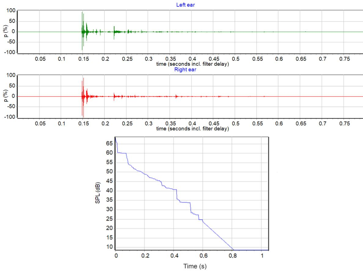
Figure 6 – Binaural room impulse response and decay curve (1 kHz) for receiver 19.
