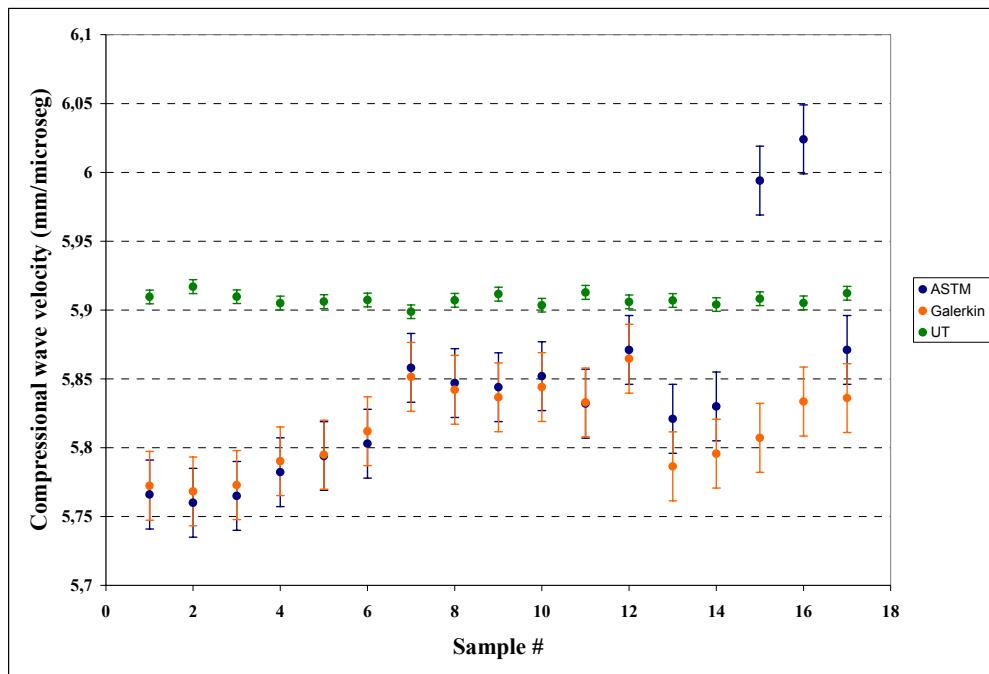
**Figure 3:** Measured compressional wave velocity by impulse excitation of vibration using ASTM standards (blue), using the Galerkin method (orange) and by ultrasonic pulse-echo technique (green)
